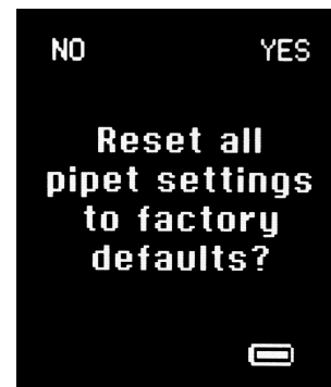
Resetting the pipette to factory settings
