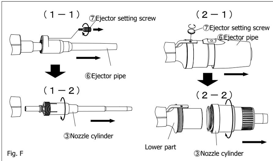
② Turn the nozzle cylinder counterclockwise to remove it, as it is screwed into the main body.
