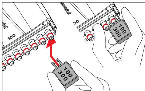
1. Push the opening of the O-ring tool (included in the delivery package) against the tip cone from the side so that the sharp edge in the opening of the O-ring tool is positioned on top of the o-ring. Do not slide the O-ring tool onto the cone!
