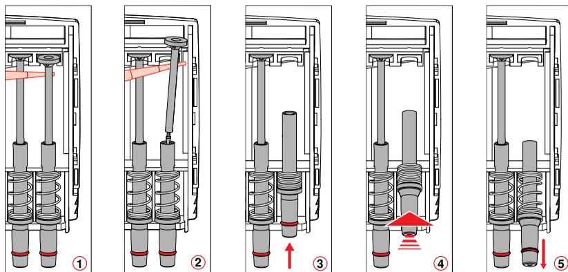
1. ① and ②: position a pipette tip under the piston and carefully take the piston off the upper rail.
