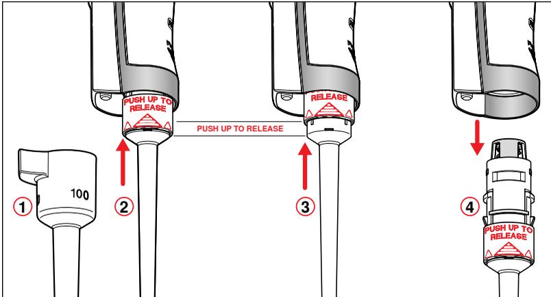
1. Keep the ejector pressed and remove the ejector sleeve ①.
