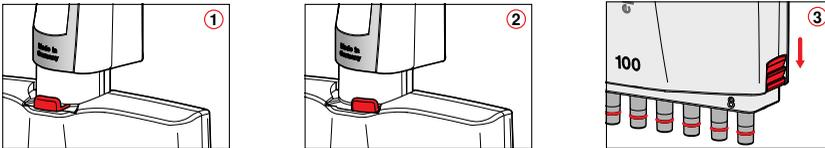
1. ① and ②: slide the lever on the lower part to the left or right.
