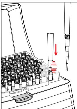
The pipette is only functional if a pipette tip has been attached. You can either attach the pipette tip by hand or directly insert the end of the pipette into a tip held in the tip storage box. If attaching a pipette tip by hand, it must be handled in such a way to avoid contamination and heating of the pipette tip.
