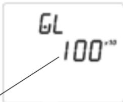
3. Select the service interval (number of pipetting cycles whereupon the pipettor alarms service)
