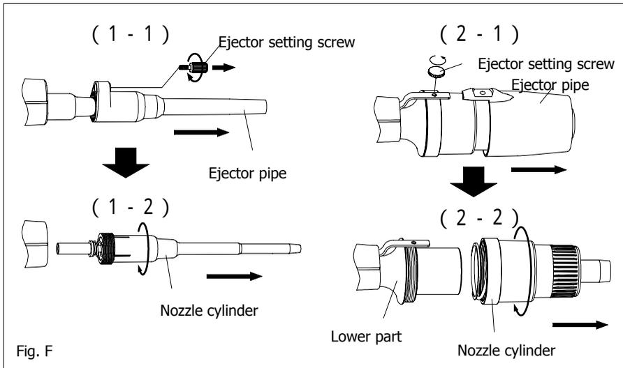
Turn the nozzle cylinder to counterclockwise to remove it, as it is screwed into the main body.
