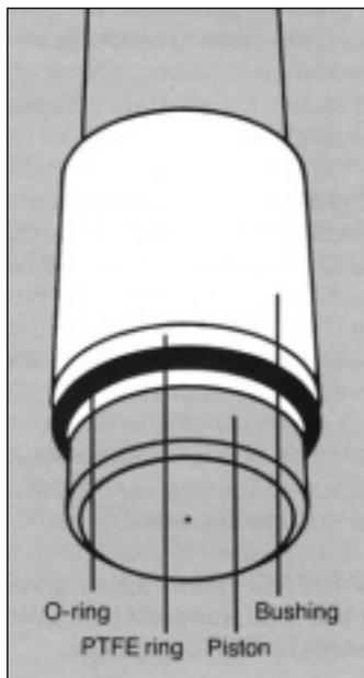
Carefully replace the shaft body on the control module, making sure that the tip ejector pin on the module engages the tip ejector hole in the shaft. Thread the retainer ring carefully back onto the control module and tighten.
