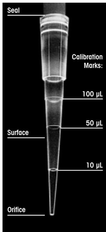
EDP2 pipettes are designed for use with RAININ-manufactured disposable tips. Specified performance of EDP2 pipettes is guaranteed only when RAININ disposable tips are used, as recommended in Section 7. Rainin Instrument, LLC cannot accept responsibility for poor performance resulting from the use of other than RAININ disposable tips.
